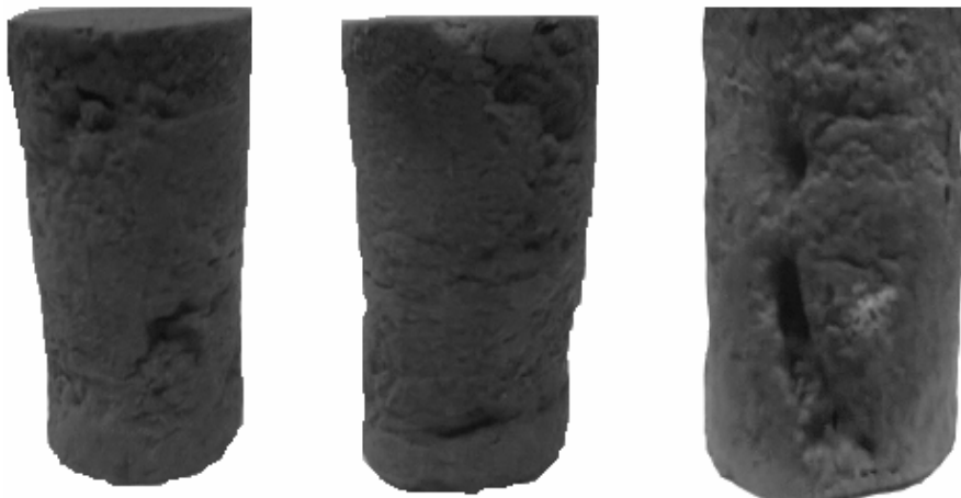
Figure 4 – Erosion in loess samples for filtration technique taking place in parallel with stratum
