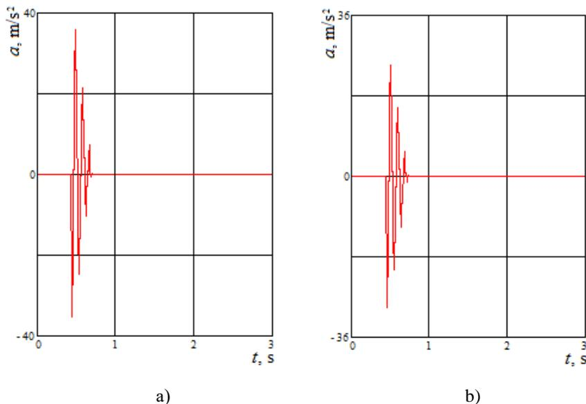
Figure 1 – The accelerations influencing the car during shunting co-impacts:
