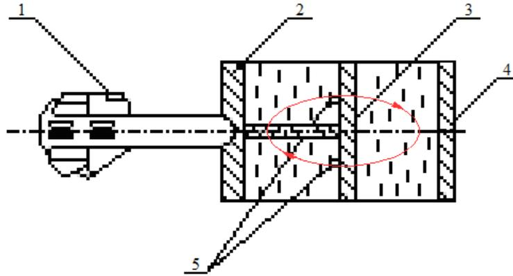
Figure 4 – The operation of the automatic coupling device considering implementation of viscous materials as springs for longitudinal forces to the supporting structure of a car body
