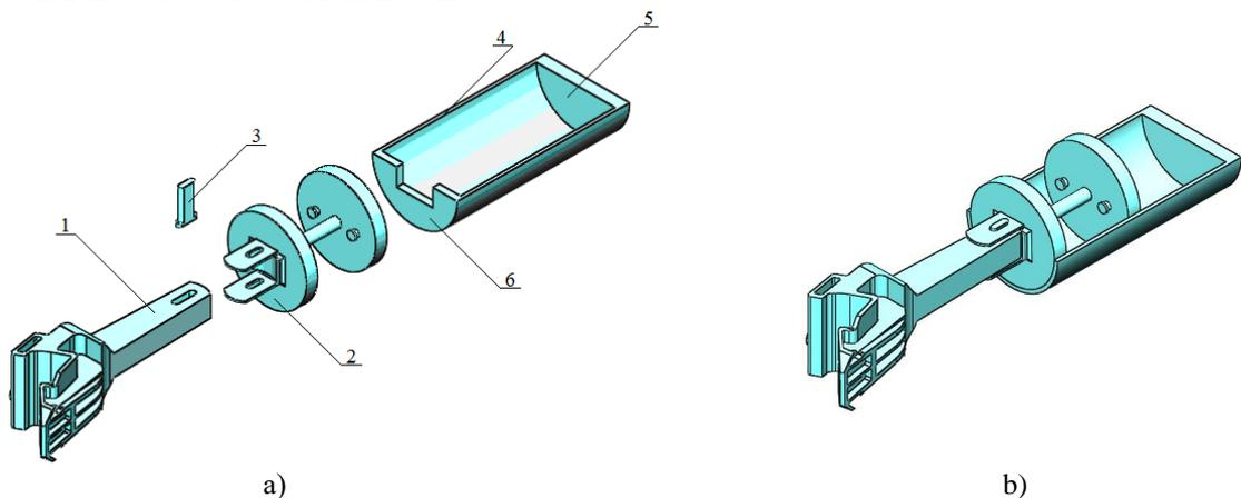
Figure 2 – Structural peculiarities of the automatic coupling device considering implementation of viscous materials as springs for longitudinal forces on the supporting structure of the car body:
