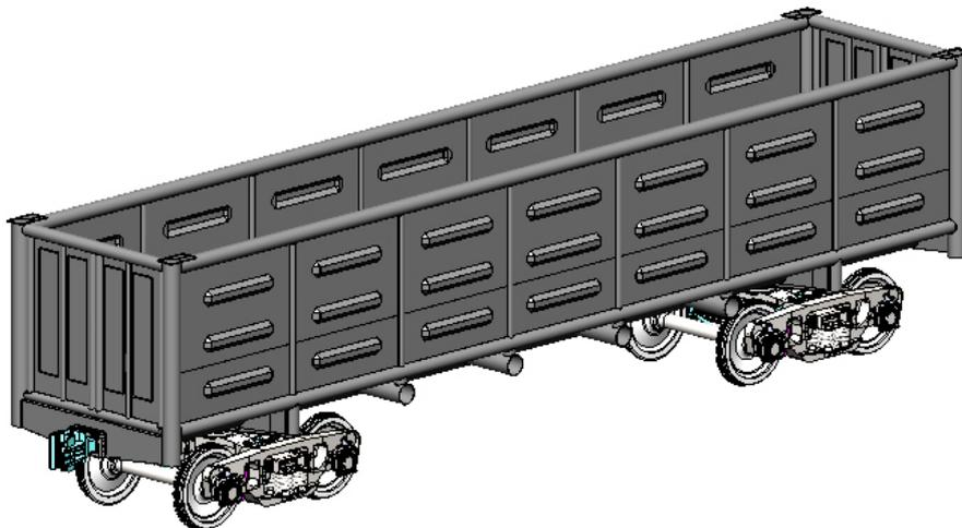
Figure 5 – The computer model of the supporting structure of the open boxcar body made of circular pipes
