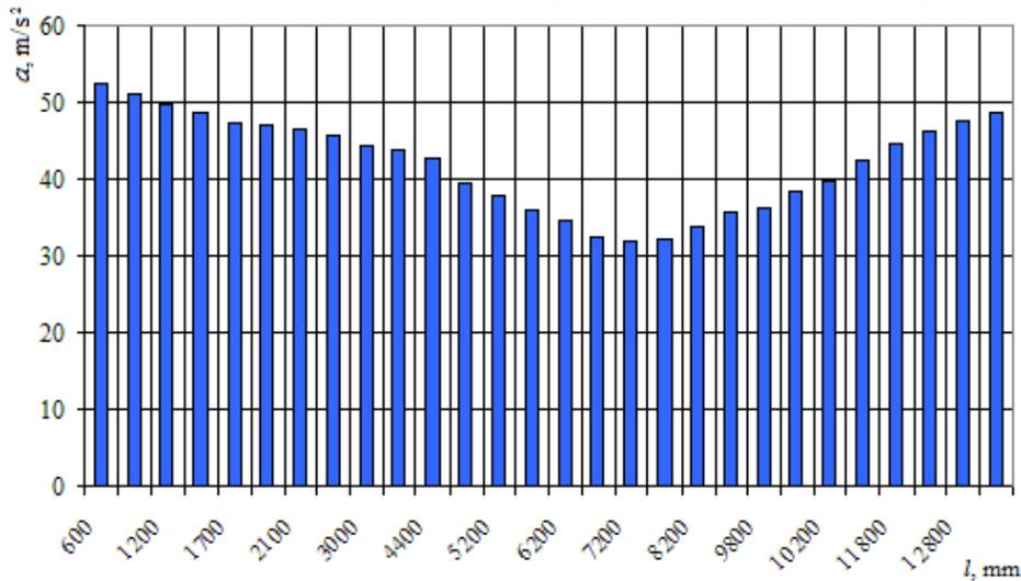
Figure 9 – The distribution of accelerations along the centre sill of an open boxcar frame under the impact force on the adapter
