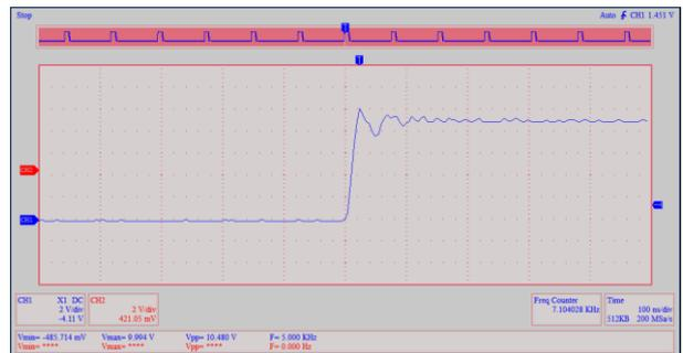
Figure 11 – Front of calibration pulse
