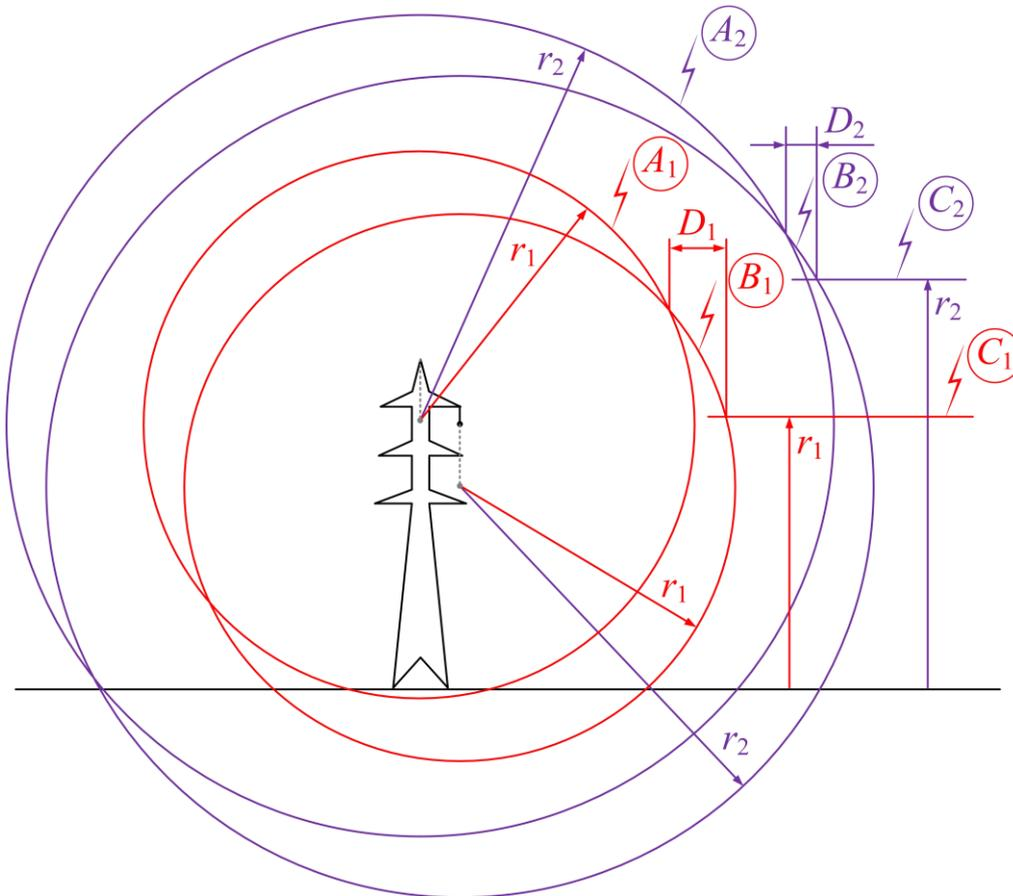
Figure 2 – Application of electro-geometric model for 36 m tall double circuit 220 kV power line tower (visualization for overhead shield wire and one phase conductor)
