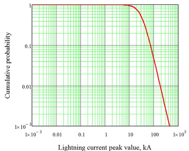
Figure 1 – Cumulative distribution of lightning current peak value in logarithmic scale on both axes
