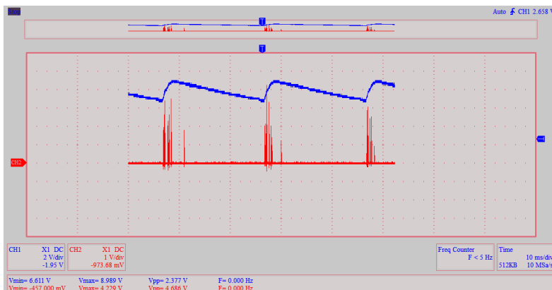
Figure 7 – Time-resolved pattern of partial discharges in moistened insulation at 9.0 kV DC ripple voltage
