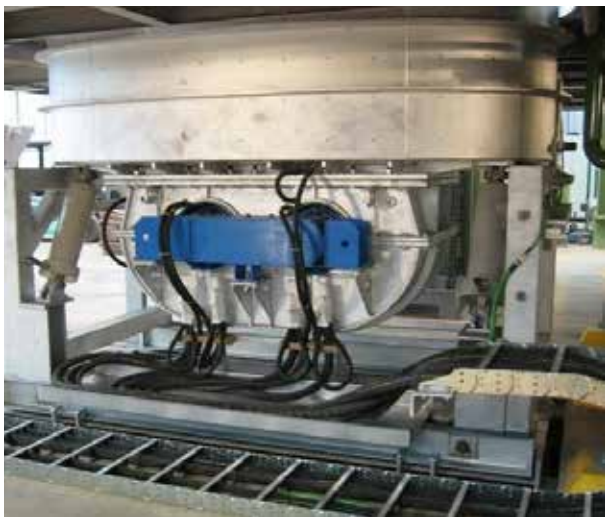
Fig. 1. General view of an induction channel furnace
